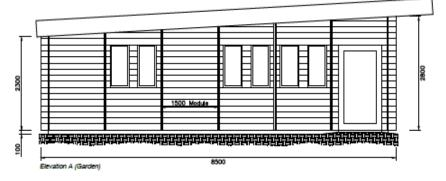
High level windows with opaque glazing to this elevation
